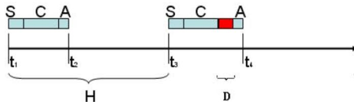
Figure 2. Jitter effect in event driven control.
