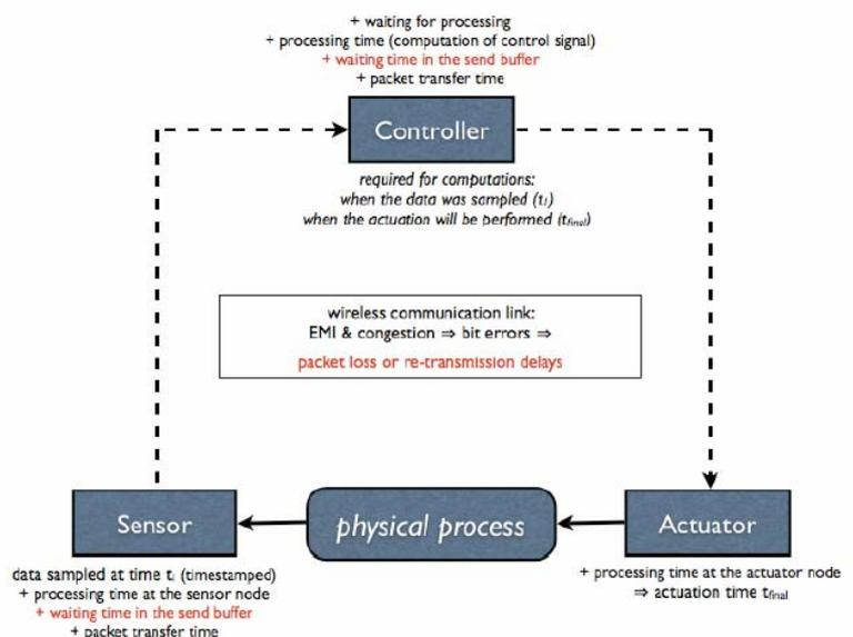
Figure 1. Sources of delay (and jitter) in the system
