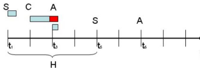
Figure 3. Jitter effect in time driven control.
