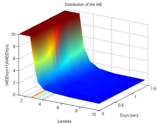
Figure 6. The IAE error changing the delay and the closed-loop time constant.
