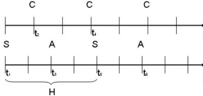
Figure 4. Delay caused by clock drift.
