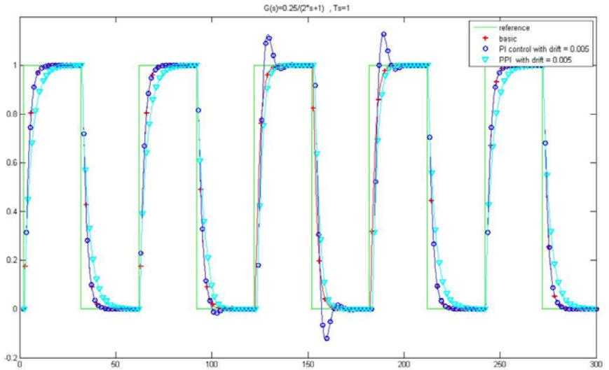
**Fig. 4. Comparison of reference tracking between PI and PPI**
