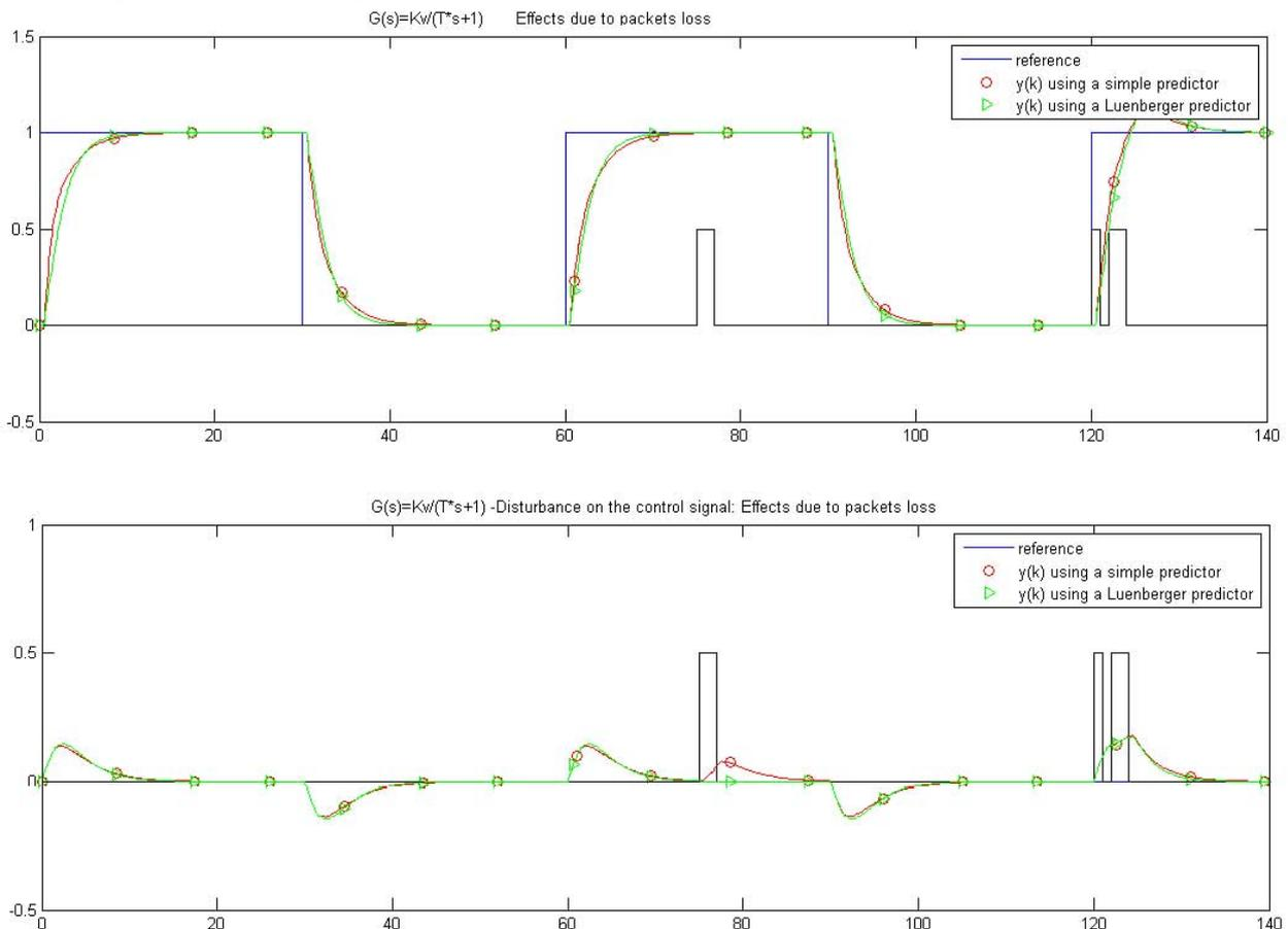
**Fig.7. The performances of predictors. (reference signal in the lower figure is null)**
