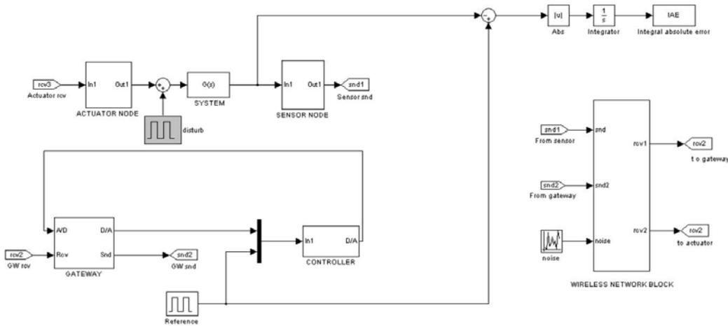
**Fig.5. Simulink model of the system with input disturbance**
