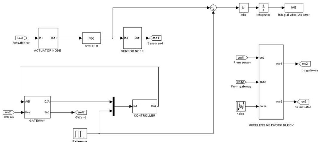
**Fig. 2. Representation of the simulated control system.**
