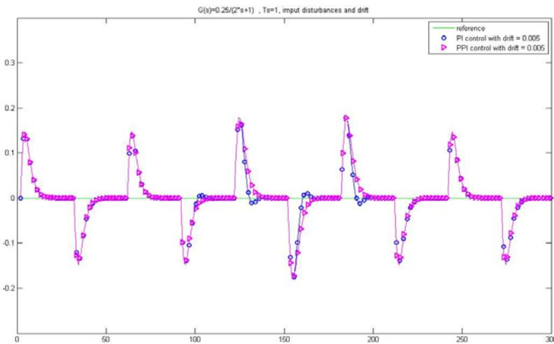
**Fig. 6. System output with disturbance and drift**
