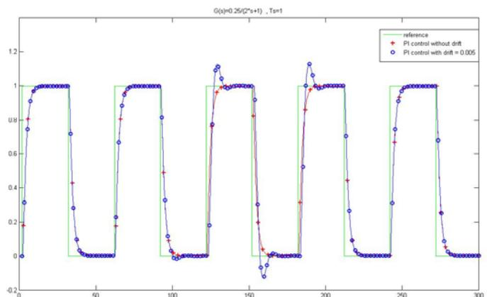
**Fig. 3. Reference tracking using the PI controller with and without drift**
